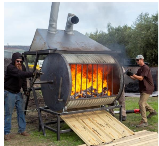
Figure 13. 4-ft diameter RoCC kiln, rear view, preparing to unload biochar. 28 February 2020
