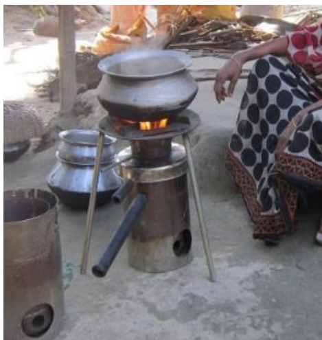
Figure 7. Indian woman cooking food on a Champion TLUD BC&E pyrolyzer cookstove (conceptually designed by the author in 2005).
